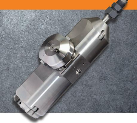
he new Torrent 50 self-rotating nozzle offers superior 3-D cleaning action for totes, tanks, and a variety of vessels. This new three dimensional nozzle is designed specifically for vessels with small openings of 6" (15 cm) or larger, and is rated for pressures up to 20,000 psi (1,400 bar), and flow rates up to 50 gpm (183 lpm).
