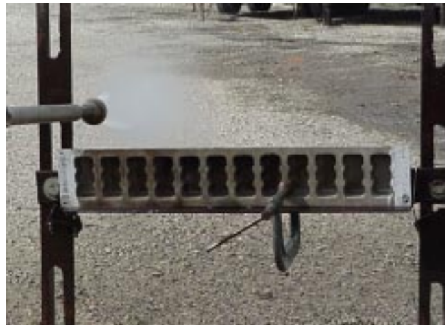
Pan being cleaned with NLB 8400A-2 rotating cleaning lance.
